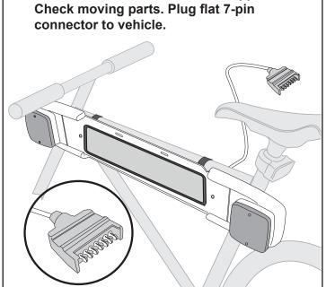
4 Secure excess cable with ties supplied.
