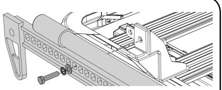
With the high lift jack securely in place, swing the clamp down over the jack arm and tighten the M10 x 30 mm Hex Screw.
