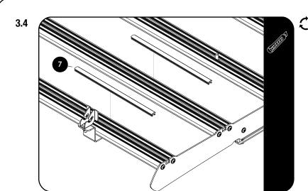
Cut the T-Slot Rubber (Item 7) into two equal lengths before inserting it into the slats T-slot as shown.
