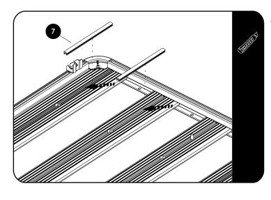
Cut the T-Slot Rubber (Item 7) into two equal lengths before inserting it into the slats T-slot as shown.
