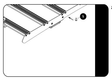
Slide the M8 x 16 Hex Bolt (Item 5) into the 3rd slat as shown.
