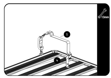
Loosely fit the Pro Tank Strap (Item 1) to the rack using the M8 x 16 Hex Bolt From 2.2 and M8 Nyloc Nut (Item 4) as shown.
