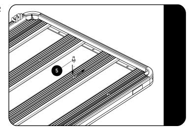
Slide the M8 x 16 Hex Bolt (Item 5) into the 3rd slats machined slot as shown.
