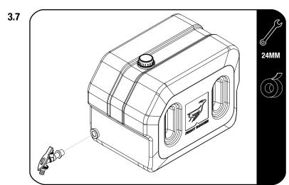
If you are fitting the tap apply thread tape to the thread of the tap.
