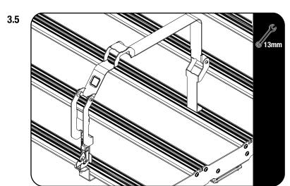
Loosely fit the Pro Tank Strap (Item 1) to the rack using the M8 x 16 Hex Bolt From 3.2 and M8 Nyloc Nut (Item 4) as shown.
