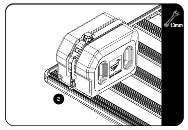
Open the Strap and place the Pro Water Tank onto the rack. Close the Strap over the Water Tank as shown.
