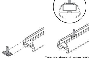
Ensure drop-&-turn bolt is aligned correctly to clamp the crossbar as shown.
