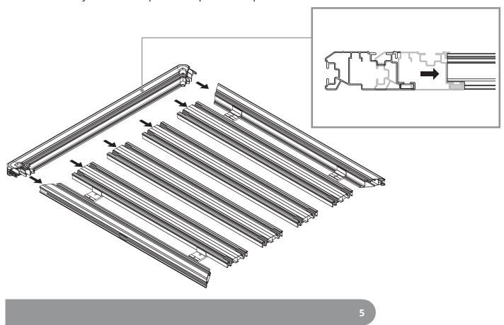
Slide the other end assembly onto the main body of the tray as shown.
