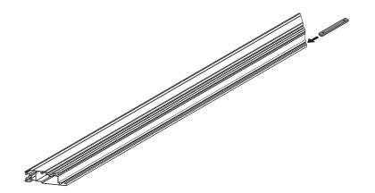
1200 wide trays = 4 per front/ rear extrusion 1400 wide trays = 5 per front/ rear extrusion
