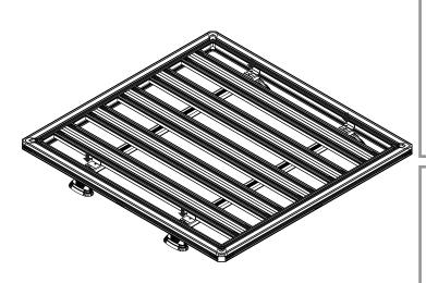
With a marker, create a reference onto the crossbars below, using each side mount block. **Do not use the centre hole** on the side mount blocks. Once selected, use the **same** hole on each mount block.
