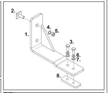
Slide the brackets into the C channel of the crossbar using the installed Plate Nuts. Tighten with a 13mm socket wrench. Check all fixtures are secure before driving.
