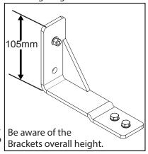
Insert the bracket assemblies into the Sunseeker as shown.
