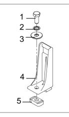
Remove the rubber buffer strip from the crossbar. Loosen the channel nut and slide the load holder T shaped section into the top recess of the Rhino crossbar.
