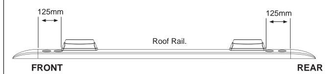
Note Vortex crossbars can be cut to length to fit this vehicle. Measure the desired length out **from the centre of the Vortex Bar** and create a reference with a marker. Carefully cut the bar at these markings using a Saw with an Alloy Cutting Blade.
