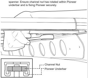
Once Pioneer Underbars have been aligned properly, tighten
