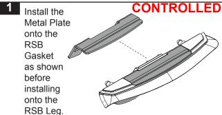
Wide end of Gasket faces toward front of vehicle. Note Left (LH) and Right (RH) for correct side of vehicle. Wide End faces forward.---
