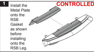
Wide end of Gasket faces toward front of vehicle. Note Left (LH) and Right (RH) for correct side of vehicle.
