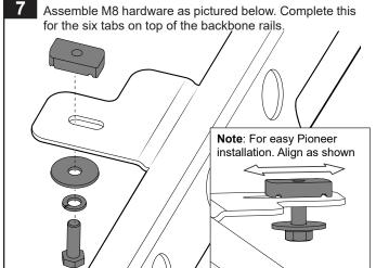
Once Pioneer underbars have been aligned properly, tighten all M8 hardware using 13mm (17/32") socket wrench or 13mm spanner. Ensure channel nut has rotated within Pioneer underbar and is fixing Pioneer securely. Tighten to 8-10Nm (6-7lbs/ft).
