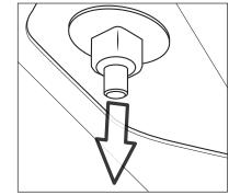
With the factory hardware removed, carefully lift the rails from the roof of the vehicle.
