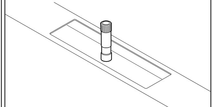
**7** Place the completed fixed mount assembly over the installed adaptors as shown.
