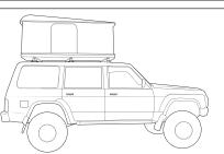
When these roof racks are to be used on a vehicle that is driven off sealed roads, the maximum roof rack load rating should be divided by 1.5. Do not forget to subtract 5kg from your maximum carrying capacity due to the weight of the crossbars and legs.
