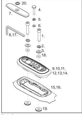
Tools Required: 5mm/6mm security allen key.10,13mm socket wrench. Flat blade screw driver.
