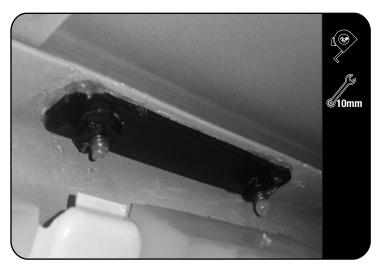
Drop the interior roof liner. Place a bead of silicone on the four nut plates (Item 13), and secure the slimsport roof rack to the nut assemblys as shown in step 2.6. This will allow easy removal of the rack in the future.
