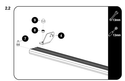
Fit the Light Bar Bracket 01 LH / RH (Item 4) for for the 40" Light Bar, using M8 x 16 Hex Bolt & M8 Nyloc Nut (Items 7 & 9). Fit the light bar and center it on the slat before fully tightening the brackets.
