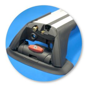
• Ensure the plastic knob is in the position shown when fully tightened.
