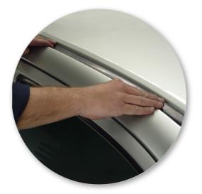
Re-install rubber ditch mould in roof channel. Remove all masking tape.
