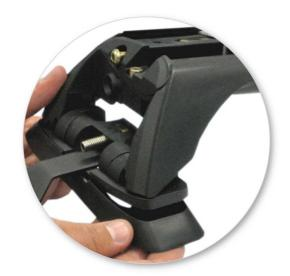
Fit rubber pads (supplied with fitting kit) to foot. Pad may vary in shape to that shown.
