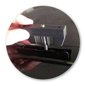
Place load support over grubscrew as shown.
