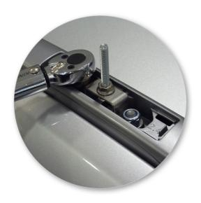
Install nuts and washers, tighten with a 13 mm socket to secure the bracket.
