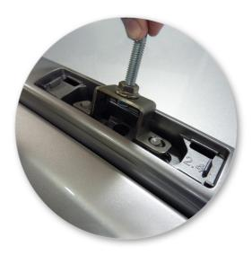
Install bracket ensuring the short leg sits over the existing nut position.
