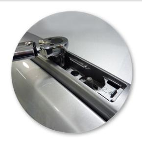
• Using a 12mm socket, remove existing nut.
