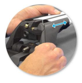
Press adjusting screw to adjust the leg positions on the crossbar.
