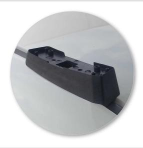
Place rubber pads (supplied with fitting kit) on the vehicle roof. Pad may vary in shape to that shown.
