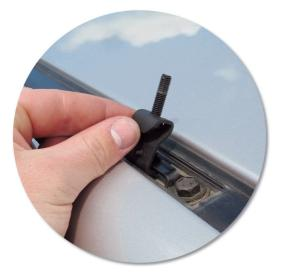
• Hook clamps into the fixed points on the vehicle.
