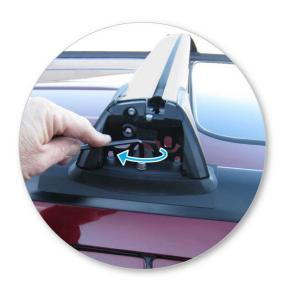
Tighten foot and cover plate down using the Hex Key.
