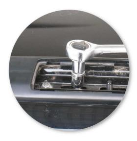
The fixed point studs have a thick layer of paint. Remove paint by using the M8 nut supplied. Use a socket spanner and run the nut down the centre stud only.
