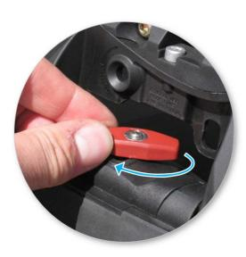
• Tighten the plastic knob. The side with the nut showing should be facing up.
