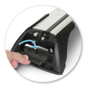
Select plastic internal block (from fitting kit) and insert into foot.
