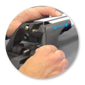
Adjust the legs on the crossbar so that they are positioned equally from the ends of the crossbar, and the clamps engage firmly on the body work of the vehicle.
