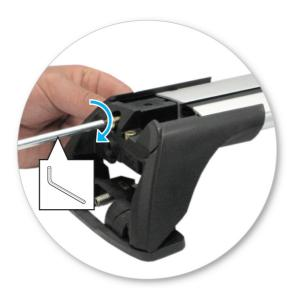
Remove plastic clamp block by gripping bar leg with fingers and push firmly with thumbs until clamp block drops out behind
