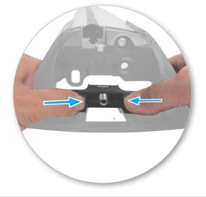
leg with fingers and push firmly with thumbs until clamp block drops out behind leg.
