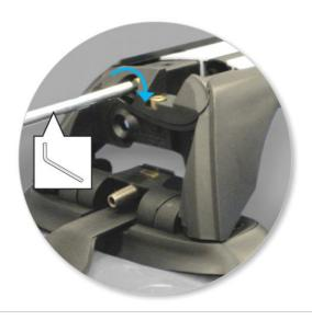
• Tighten adjusting screw to 5 Nm.
