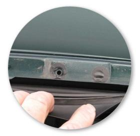
• Pull back rubber seal to expose fixed points on vehicle body.
