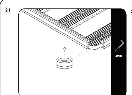
Start with removing the front right-hand Corner piece with a 4mm Allen Key.
