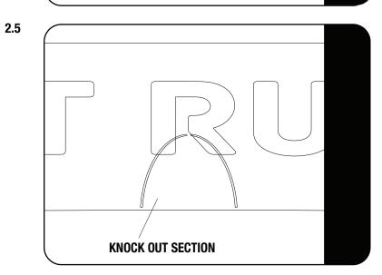
If your vehicle has a Roof Antenna which interferes with the Wind Fairing touching the roof. The knock out section can be removed.
