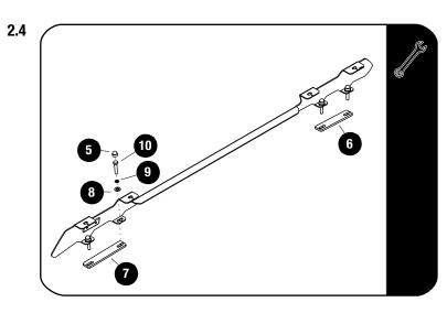
Place a bead of silicone down the threads of each bolt before inserting.
