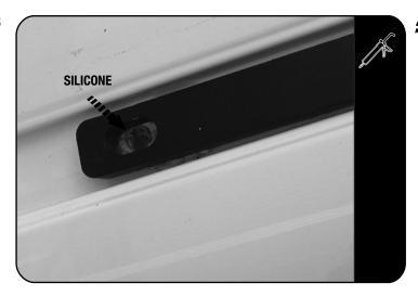
Clean the area around the holes in the vehicle's roof using a rag and methylated spirits or denatured alcohol. Place some silicone around each hole in the vehicle's roof.
