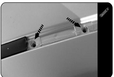
Looking at the Ditch, where you have just removed the Ditch Moulding, locate the four Threaded Mounting points in the vehicle's roof and remove the Protective Tape covering them.
