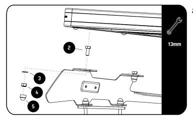
Fit your roof rack to the Foot Rails using M8 x 20 Hex Bolts, M8 x 16 x 1.6SS Flat Washers and M8 Nyloc Nuts (Items 2, 3 & 4) as shown.
