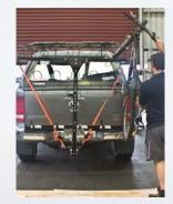
2. To load a bike, facing the rack stand on the right-hand side of the bike, taking the right handle-bar grip with your right hand, and right-hand rear triangle with your left hand lift the front wheel into the basket, pushing the wheel to the front making sure it is resting on the top rail. Lower the back wheel onto the mid rail wheel rest.
