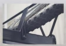
3. Loop the bungee around the front wheel rim and secure to the button at the front. If the Cam Straps are used, wrap the strap around the front wheel rim and pull tight.
