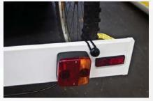
6. (Optional) to attach the Dirty Possum Light Bar, push the bungee ball loop through the orifice and around an appropriate back wheel, securing to the ball on the front of the light board. The light board comes with a 7-pin large round plug, if necessary, use an adaptor or plug straight into your vehicle socket.
