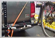
4.Ensure the left-hand side crank arm is pointing downwards, loop the cam strap over the pedal spindle (hard against the crank arm). If necessary, adjust the midrail to the centre of the bike wheel.
