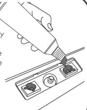
ASSEMBLE PIVOT BRACKET TO RUGGEDLINE
