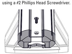
Secure using Plastite Screw. Tighten
