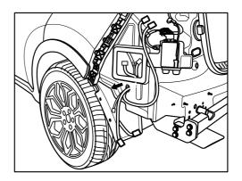
22. Inside the LHS rear quarter vent cavity, secure the trailer patch ground ring terminal (1) to the vehicle grounding point (2).
