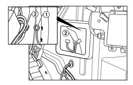
23. Connect the trailer patch connector (1) to the ECU (P/No: 04826) (2). Locate a suitable area on the sheet metal (3) where the ECU will be mounted and clean with an alcohol wipe (not supplied). Remove the backing from the back of the ECU and mount the ECU (2) onto the sheet metal area (3). Ensure the ECU is mounted with the connector pointing downwards.
