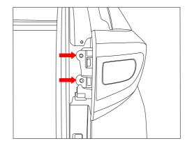
4. In light cavity, remove 2 x Scrivets.
