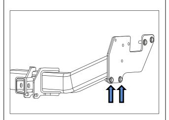
On the factory step, remove the 2 x M12 Set Screws securing the mounting bracket to the step body.
