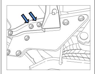
Fit all remaining fasteners to secure the Towbar. Torque all fasteners to the following specification:
