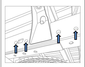
Loosely secure sidearm by using 2 x M12 x 1.25P Set Screws with Flat Washers on the most forward to mounting points on the vehicle. Repeat for opposite side.
