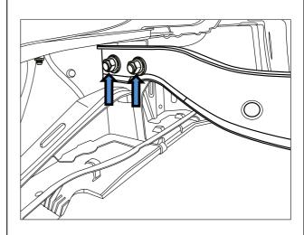
Re-attach the mounting bracket with the 8MM spacer supplied. Repeat for opposite side.
