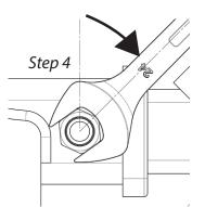
Fig 4. Tightening of Smart Pin Nut
