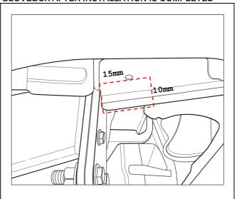
8. Loosely insert 1 x M12 x 1.25P Set Screw with Flat Washer to the second last rear mounting mount point on the vehicle. Allow the Set screw to be partially inserted into the thread on the vehicle. Repeat for opposite side. Then re-attach the factory step and insert the remaining 1 x M12 X 1.25P Set Screw with accompanying washer.
