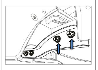
It is recommended to clean the thread 4 mounting points with a M12 x 1.25P Tap to rid female threads of paint. This will allow ease of fitment for supplied fasteners.
