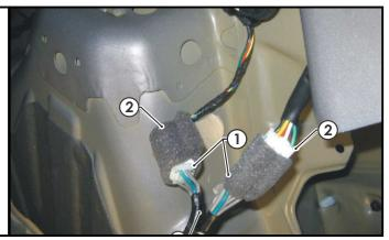
Route the 'ORANGE' power wire (1) along the existing vehicle harness towards the front of the vehicle.
