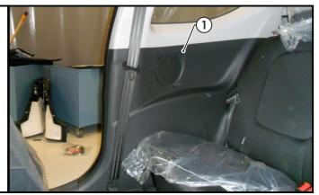
8. Remove the RHS seat trim (1) by first removing the two fasteners (2).
