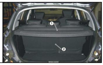
3. Remove the luggage compartment rear trim (1) by first removing the two clips (2).
