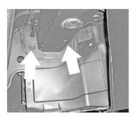
**6.** Remove 2 Scrivets from top and bottom tabs, to remove the Impact Beam, with the tabs. Repeat the step on the other side.
