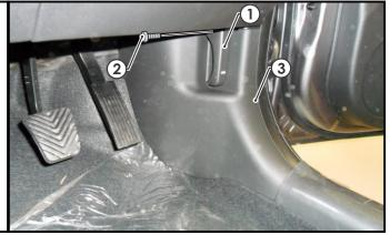
**12.** Remove the lower dash board trim **(1)** to gain access to the fuse panel.
