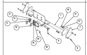
Figure 4 – Fit the towbar
