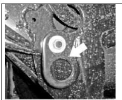
Figure 2 – Remove the shipping hook.
