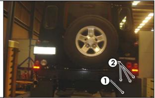
2. Underneath the RHS of the vehicle remove the panel cover (1) by first removing the two fasteners.
