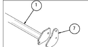
Figure 3 – Fit the End Plates.
